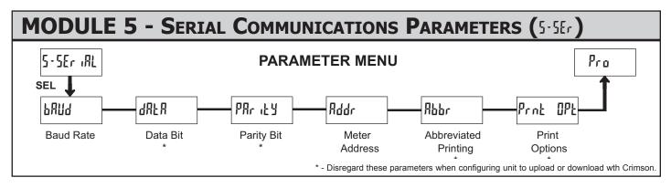
Module 5 is the programming module for the Serial Communications Parameters. The only parameters of concern when utilizing the CUB5USB programming option card to communicate with Crimson 2 programming software is the Baud Rate and Meter Address. The Parameters are only accessible when an optional CUB5USB, RS232 or RS485 serial communications card is installed in the meter.
